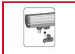
Manual release located on the bottom side of the motor
