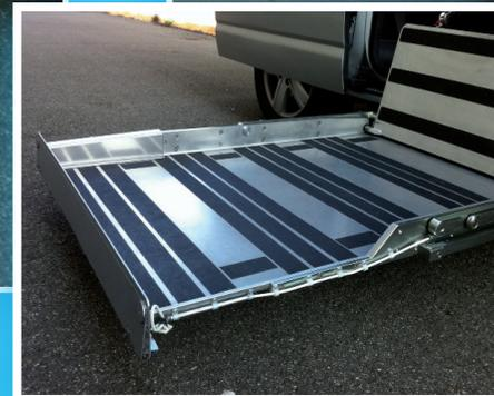
*The F900 is a retractable, completely automatic underfloor lift made in stainless steel and aluminium to be fixed in the side of the vehicle. Thanks to the extremely slim dimensions of the cassette F900 can be mounted on a wide range of vehicles for people transportation.*
