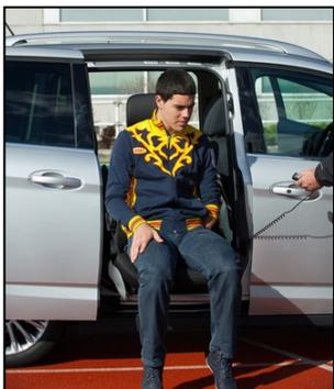
The **Turny Orbit** is a fully automatic, swivel seat where all movements are operated by the hand held remote.
