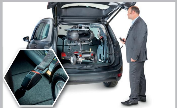
**4** The seatbelt restraint ensures your mini scooter or wheelchair is safely stowed
