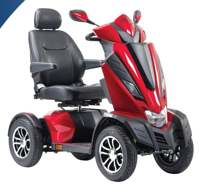
Following the success of our Cobra scooter we've developed the new King Cobra. This offers an evolved dynamic design, generous spaciousness, a 50km range and a maximum weight limit of 200kg.
