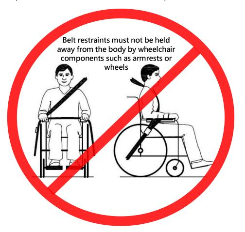
Illustration of improper belt-restraint fit
