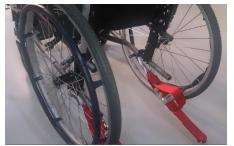
Fitting the Rear Restraint
