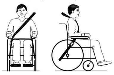
Illustration of proper belt-restraint fit
